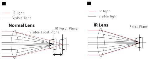
Out of focus caused by focal plane difference
